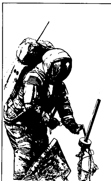
Alignment Of Passive Seismometer
