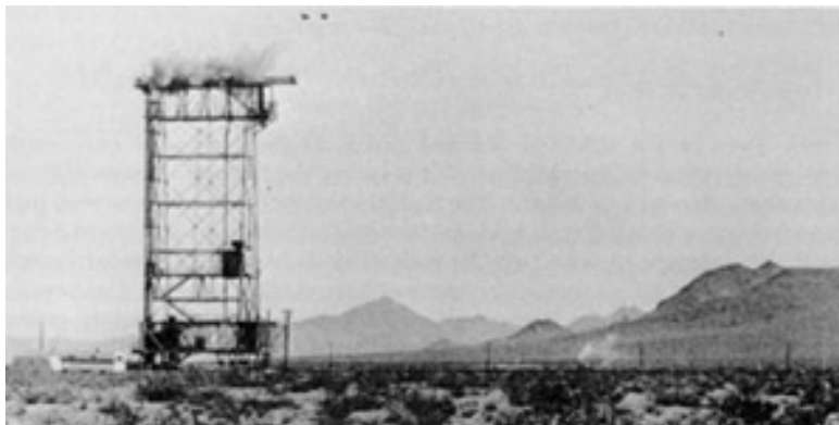
Figure 89. Simulated off-the-pad ejection test No. 13 at U.S. Naval Ordnance Test Station, China Lake, California. (NASA Photo No. 65-H-197, released Feb. 12, 1965.)
