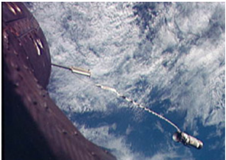
Figure 131. The Gemini Agena target vehicle tethered to the spacecraft during the Gemini XII mission. (NASA Photo No. 66-H-751, released Nov. 16, 1966.)
