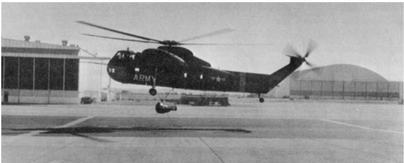
Figure 43. Gemini paraglider half-scale test vehicle slung beneath an Army helicopter at the beginning of the second deployment flight test. (NAA-SID Photo 277/4, Jan. 4, 1963.)
