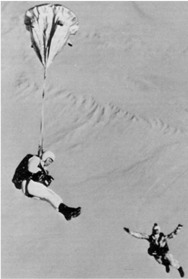
Figure 65. Jump test of the 36-inch ballute with dual suspension at the Naval Parachute Facility, El Centro, California. The second figure is a free-falling photographer with a camera mounted in his helmet. A second observer jumped later and took this picture. (NASA Photo 64-Gemini-120, released Dec. 18, 1963.)
