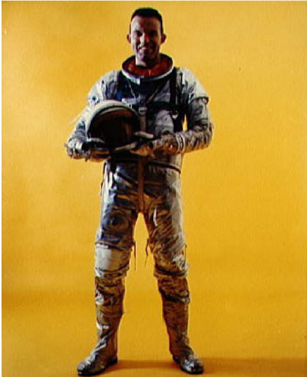
Figure 67. Flight pressure suit of astronaut L. Gordon Cooper used in MA-9, 22-orbit mission. Compare with flight pressure suit of astronaut Alan Shepard in MR-3 suborbital flight in figure 37.
