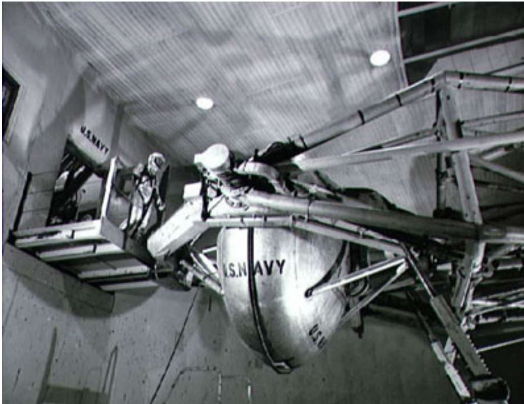
Figure 14. Human centrifuge at the Navy's Aviation Medical Acceleration Laboratory, Johnsville, Pennsylvania, used in Mercury astronaut training program.
