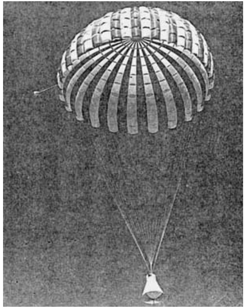
Figure 18. Main 63-foot ringsail parachute.
