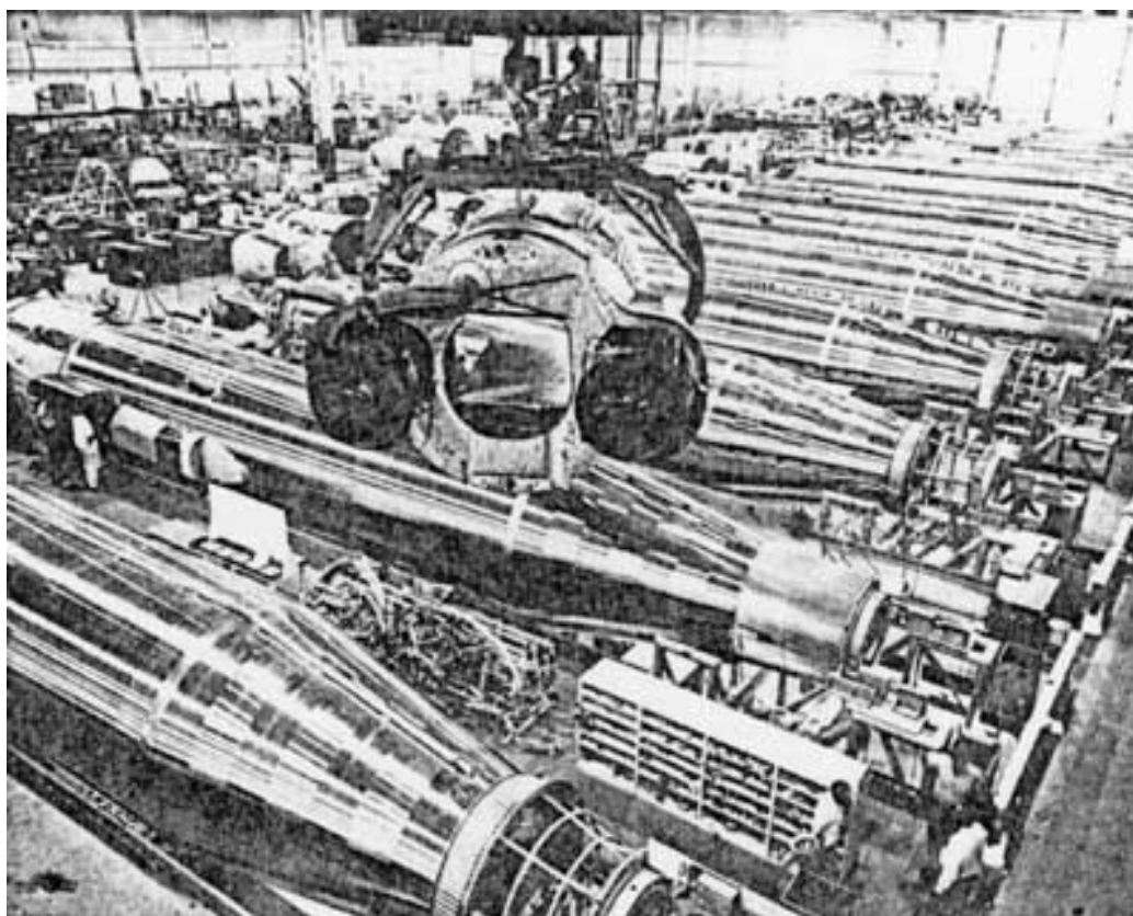
Figure 57. Production of Atlas launch vehicles at Convair Astronautics plant at Sorrento, Calif.
